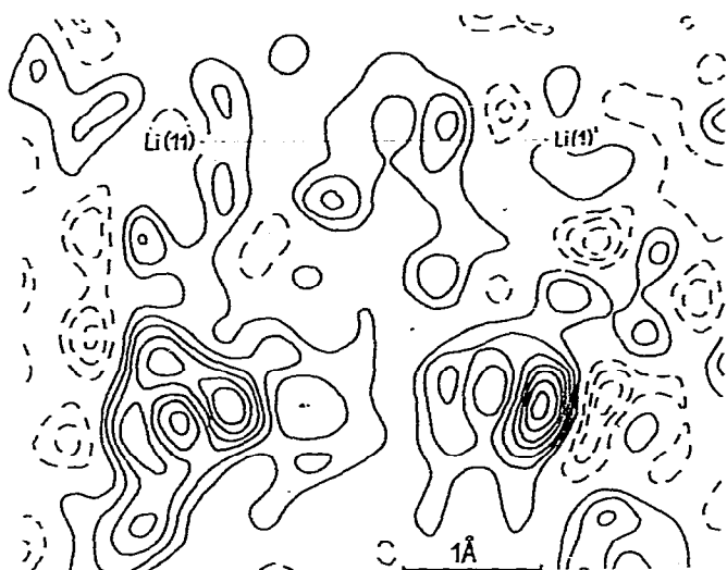
Fig. 6. F_0 - F_c synthesis section through the atoms Li(11)—L(1)' and the centre of the cluster. The inter-sections of the two lateral tetrahedron faces with the map are marked by thin dashed lines. Contours as in Fig. 4.
